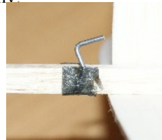
Unused sub "Blackie" shows off simple wingmount. Slide fore and aft, shim if required. Two bearings in nose, front and rear, about 1 1/2 degrees down and side. Also, all rear hooks are forward of fin, bar one model, for comparison purposes.
