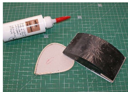
The former provides some protection for the balsa during initial (soft) sanding.
