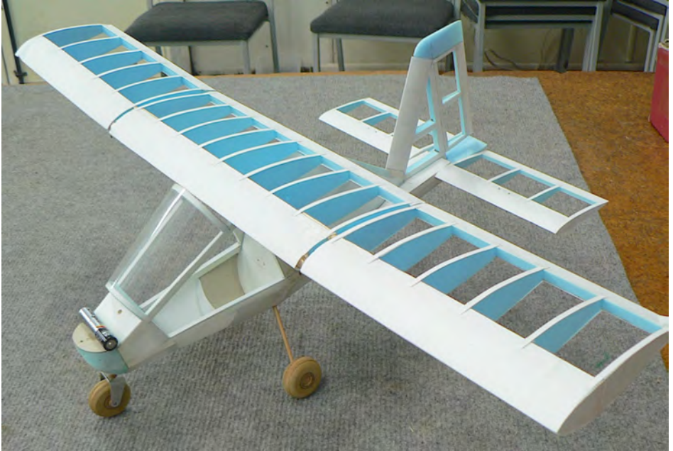
Above: Tony's concept model for a full size microlight aircraft that shows wing ribs sliced off from a common foam form.
