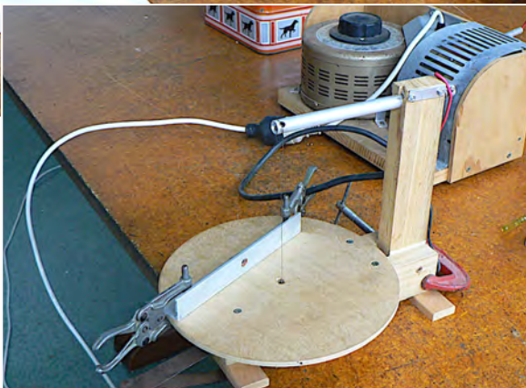
Above: Cutting a 1.5mm slice of foam from the polystyrene block, against a 100mm x 100mm aluminium angle plate.
