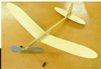
Above: Tony's concept model for a full size microlight aircraft that shows wing ribs sliced off from a common foam form.
