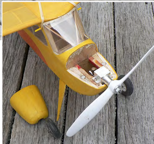
Above: The Terrier is a simple cabin model of easy and light construction. Covering is doped but unsprayed tissue.
