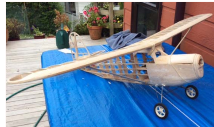
Left: Paul Evans's Shavrov Sh-2 is an unusual free flight scale amphibian, destined for electric power.
