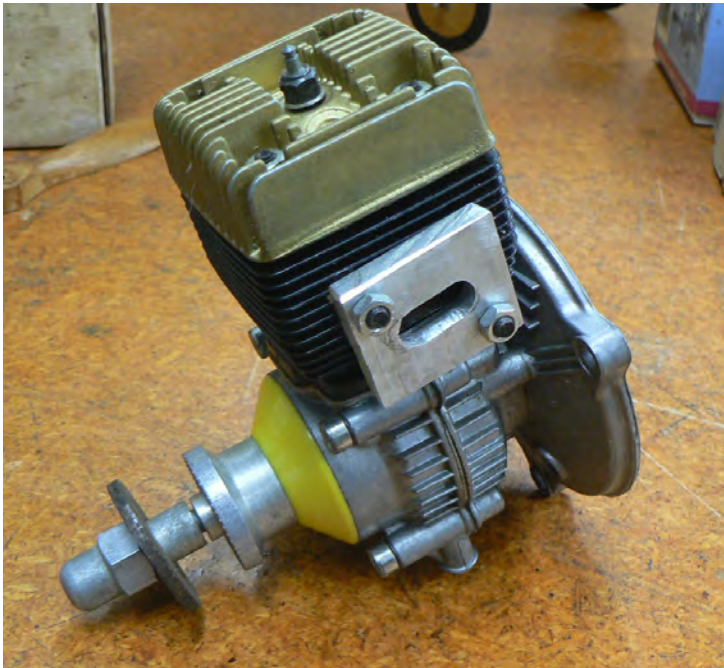
Left: Largest engine on the table, Charles Warren's Italian Tartan 1.32cu in (21cc) glow engine.
