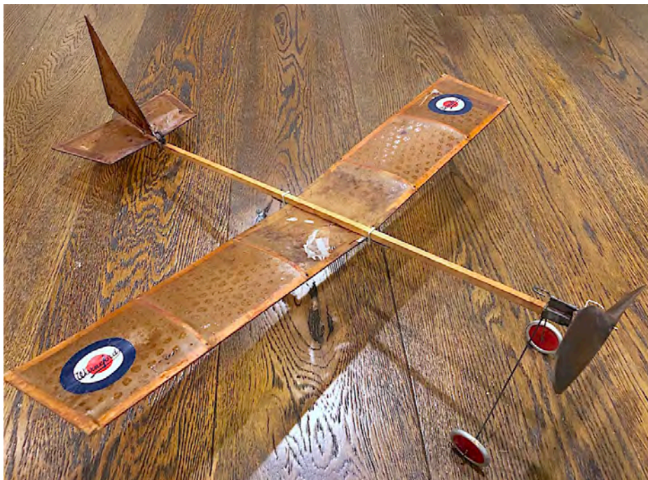
A veteran Warneford Stick Tractor oiled silk covered rubber powered ARF, first marketed in the UK in 1928 and brought to the June meeting by Mike Mulholland (see p.8). (Photo: Mike Mulholland).
