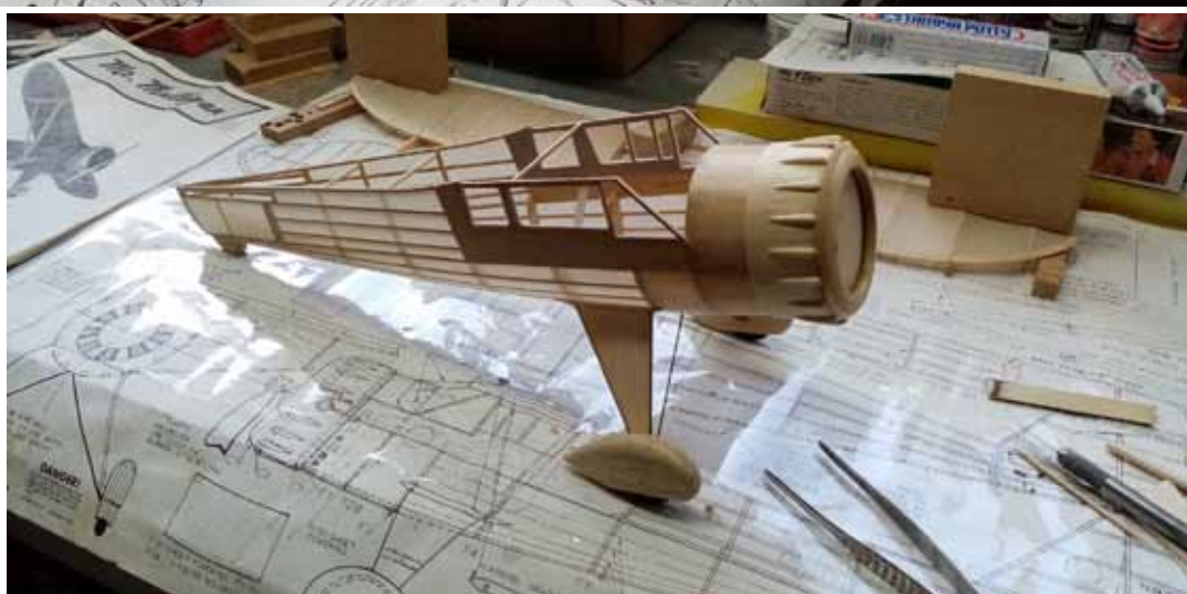
ABOVE: The view before painting showing the main stumbling blocks, the wheel spats and pesky cowl detail.
