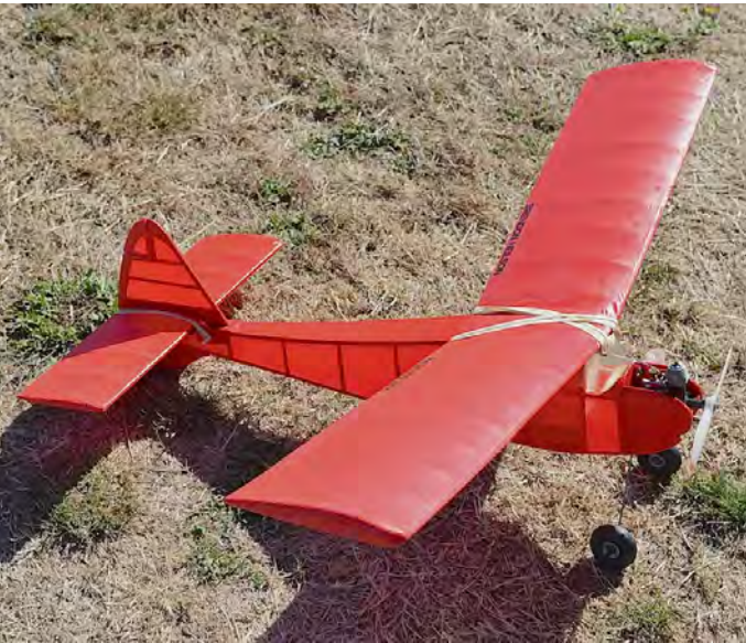
Above: Brendon Neilson's E70, backlit and showing the many lightening holes made to save weight. Photo: Ricky Bould
