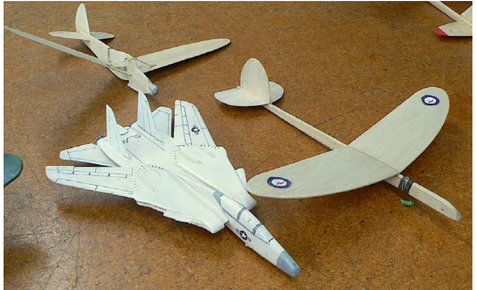
Top: George Fay's replica of the original American Junior Army Interceptor folding wing glider designed by Jim Walker, with wings that unfold instantly under the rubber bands tensioning them as the model is launched. He also brought another swing-wing, an F14 Tomcat fighter of his own design and also a more conventional looking catapult or hand launched glider.
