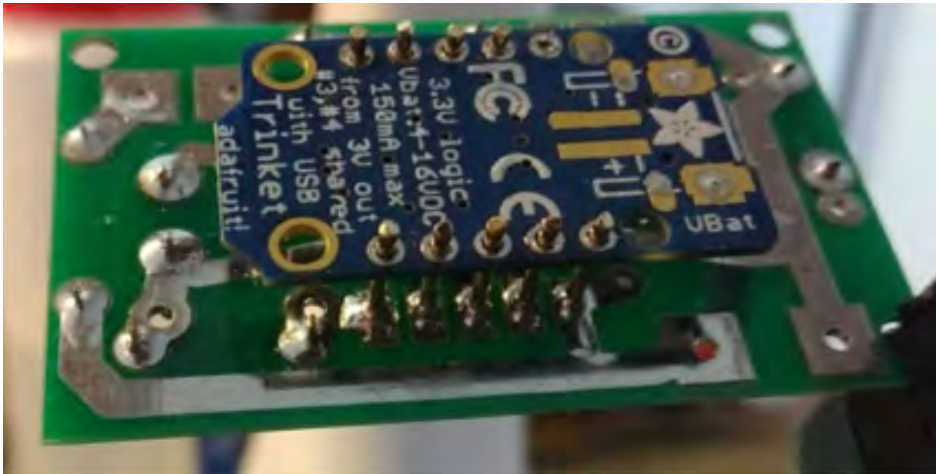
Above: Correct orientation of trinket when attaching to the pcb.
