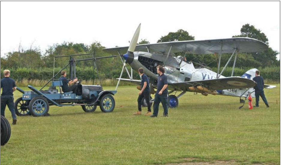
Above: Out on the field, using a Hucks starter on the Hawker Hind.
