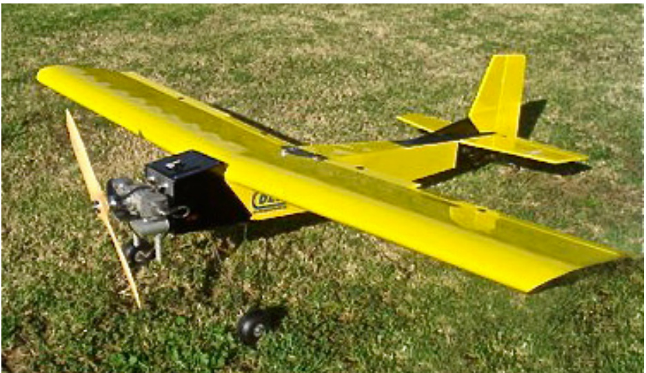
Above: Stuart Ward's Greenly Towplane powered by a DLE 60cc Twin Petrol engine.
