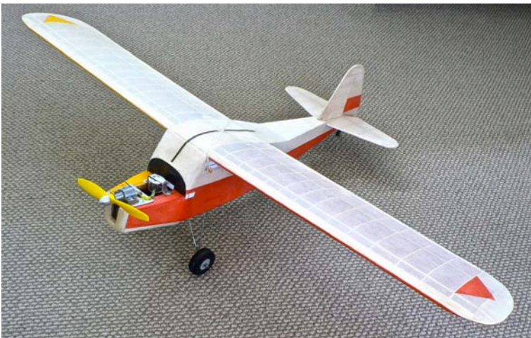
Left: The Austerboxy, purpose-built to experiment with trim set up. Also has an ED Hornet diesel for power.
