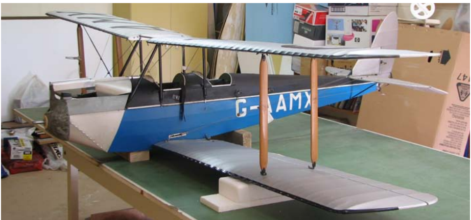
Above left: New engine mount and tank bay installed. Above right: Greater damage to upper wing repaired while attached to strut fittings. Below: Gypsy with wings back on.
