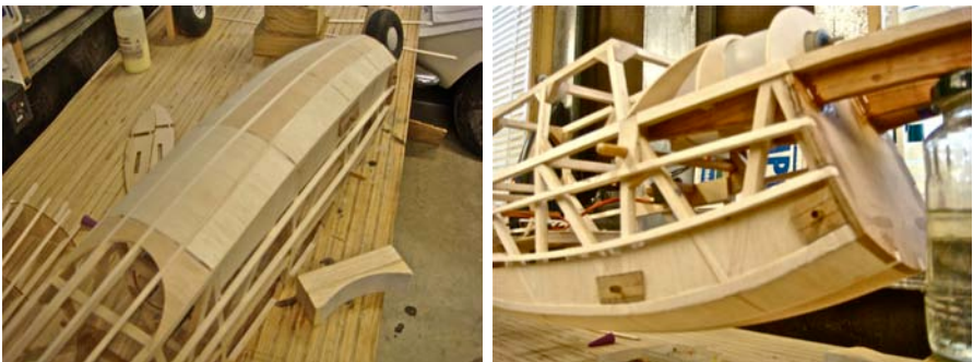
Above: Views of in-fill in the forward fuselage. Note the curved sanding block in the left hand view.
