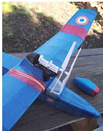
(More from Rob) Smith A modified KK invader, masquerading as a French flying boat. Built as a test bed for the contra rotating twin drone motor. Built from a modern Ripmax kit, the wood in this kit was worse than any I ever saw in the 50s so hard you couldn't stick pins thru it!!!. The only saving grace was the laser cutting which was excellent.
