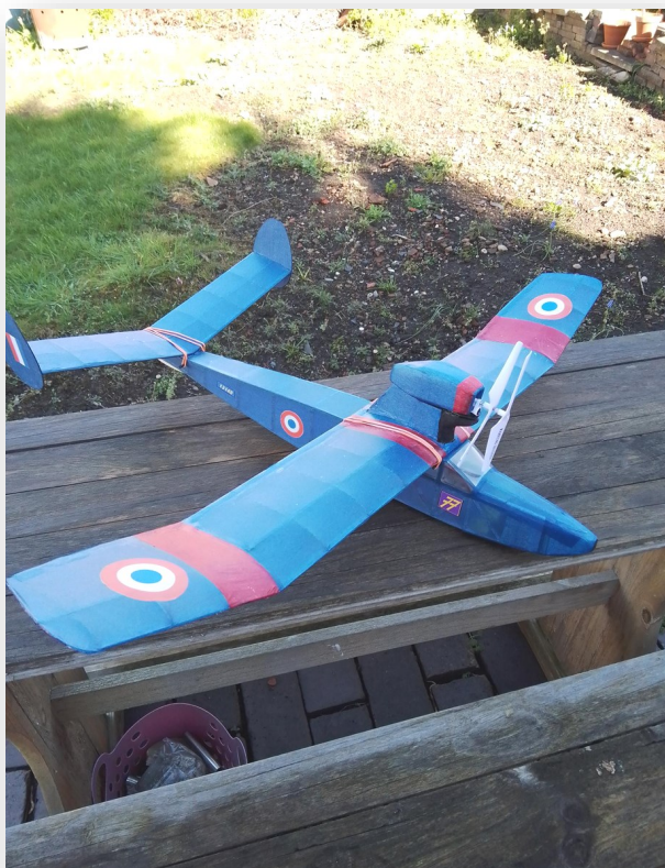
(More from Rob) Smith A modified KK invader, masquerading as a French flying boat. Built as a test bed for the contra rotating twin drone motor. Built from a modern Ripmax kit, the wood in this kit was worse than any I ever saw in the 50s so hard you couldn't stick pins thru it!!!. The only saving grace was the laser cutting which was excellent.
