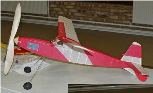
“Gypsy” built from VMC kit. Light and simple. Awaits the 8oz Wakefield event on Sunday of Nationals. Polyester covered, Spencer Willis prop.
