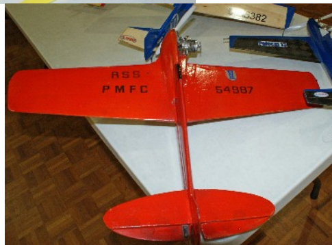
Peter Adams’ Teachers Pet, mylar covered fuselage as well as tail. 30% increase in tail area simplifies trimming. Tracker fitted to reduce the length of Peter’s countryside walks.
