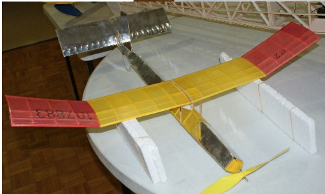
Roger Silcock’s Mike Argander Special, a 45 year old Goodyear racer. Now converted from glow to diesel: recent repairs with glass fibre . Once timed at 112mph with ST15 on board. Roger is keen to fly it again.
