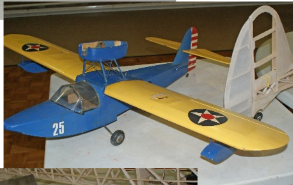
Peter Adams’ Teachers Pet, mylar covered fuselage as well as tail. 30% increase in tail area simplifies trimming. Tracker fitted to reduce the length of Peter’s countryside walks.
