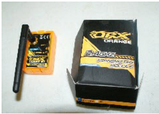
RF Module, £35, makes a 2.4 Tx. Remember Tx and Rx should be of the same make.
