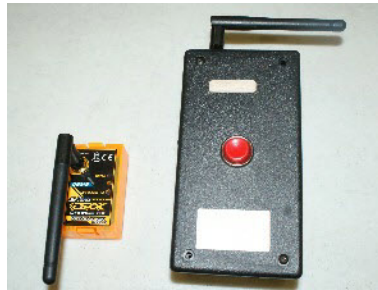
RF Module, £35, makes a 2.4 Tx. Remember Tx and Rx should be of the same make.
