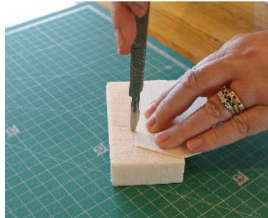
Sharon Ashmole demonstrates the non-crush slotting technique. Soft base is loft insulation
