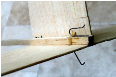
Andy's Cloud Tramp. (Several years of use caused damage to the wing roots, so harder wood has been spliced in at the trailing edge.)
