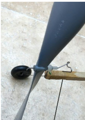
(Left) Nose plug, Teflon washer and Peck Polymers prop. Note "S" or "Z" hook and simple free wheel on prop shaft.
