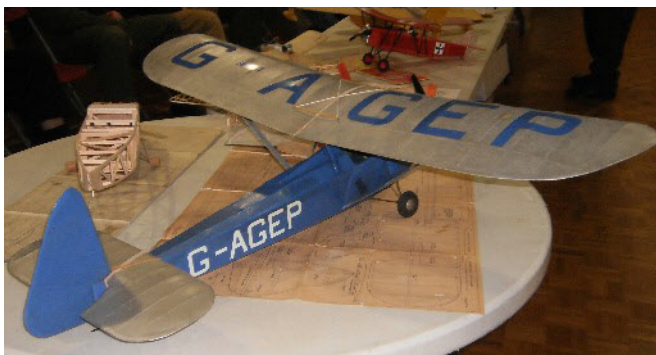
Martin Skinner's Luton. Minor. Despite grumbles from modellers elsewhere, it flies well as did the Editor's. Motor is a ZA 92 (0.92 c.c.) Dated 1962, also known as the ZA Griffon. Chosen because of its price: just 42/-
